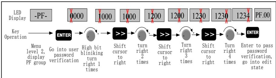
Fig. 5-15-2 Flow chart of user password unlocking
