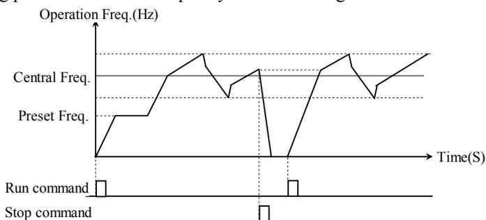
Fig. 5-6-2 Wobble frequency start: continue to operate at the frequency and direction before it stops
