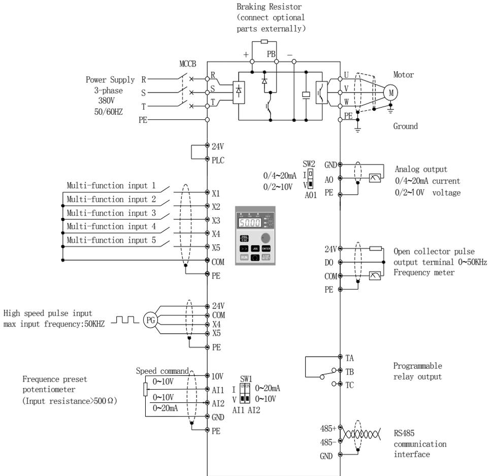
Fig. 2-34 3R75GB/31R5PB~3004GB/35R5PB Wiring diagram
