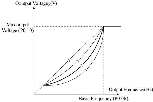
Fig. 5-0-2 Torque-reducing curve
