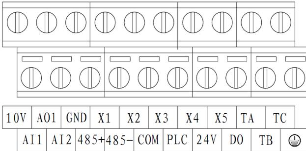
Fig. 2-12 S21R5GB~3004GB/35R5PB Arrangement of Control Circuit Terminals
