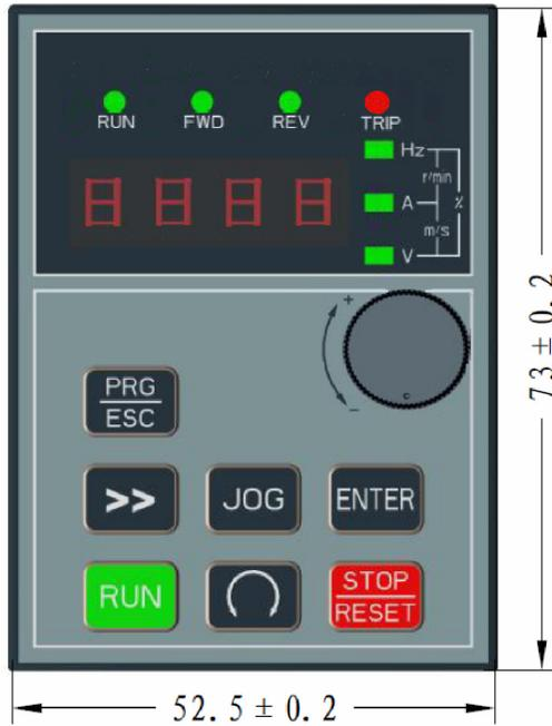
Fig. A5-1 Keyboard Mounting Size of S2R4GB~3004GB/35R5PB
