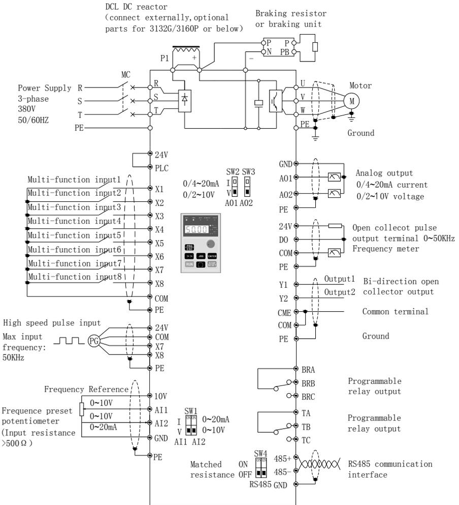
Fig. 2-36 3018G/3022P~3500G Wiring diagram
