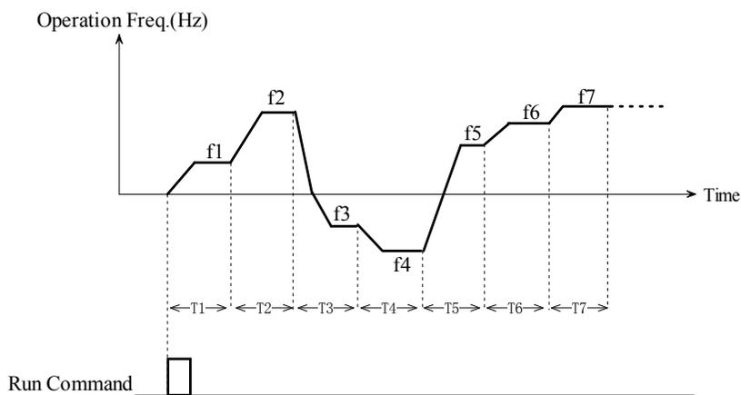
Fig. 5-5-2 Holding the frequency after single cycle
