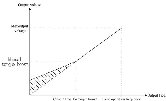
Fig. 5-0-4 Manual torque boost diagram
