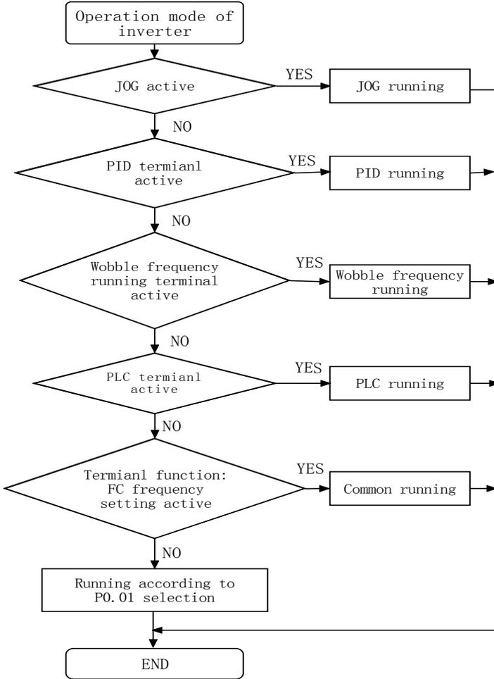
Figure 3-8 Operation modes switching of inverter
