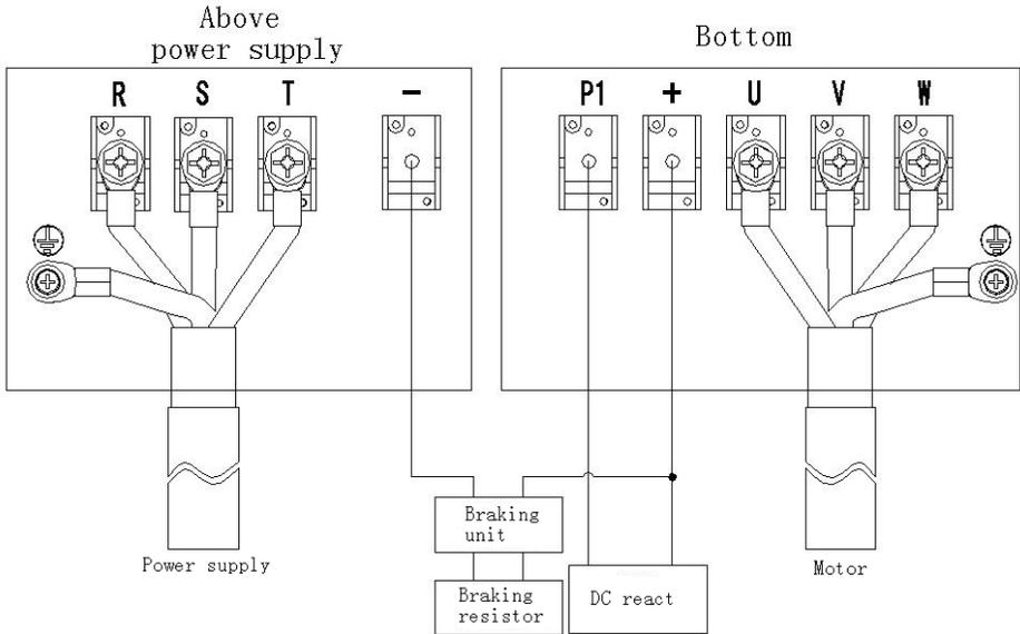
Fig. 2-8 3400G~3500G Main Circuit Wiring
