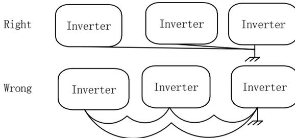
Fig. 2-9 Earthing Connection Method
