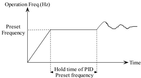
Fig. 5-7-2 PID preset frequency operation
