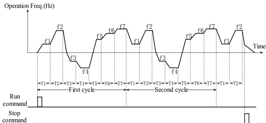
Fig. 5-5-3 Continuous operation of PLC
