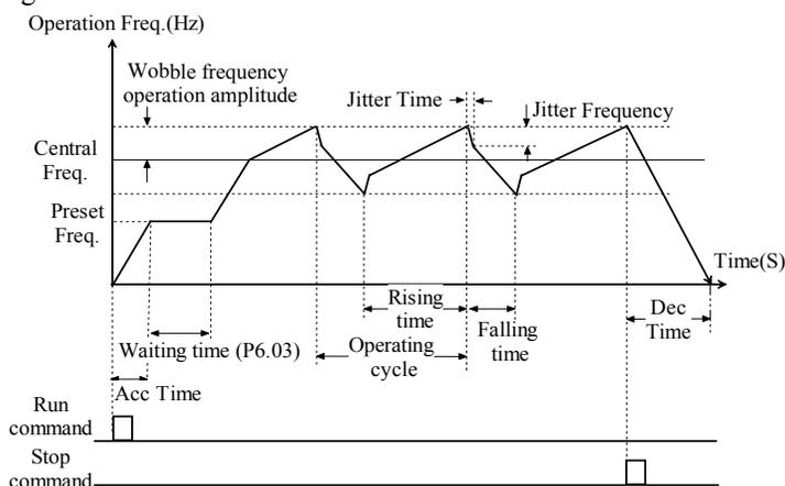
Fig. 5-6-1 Wobble frequency operation diagram
