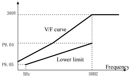
Fig. 5-9-2 Energy saving voltage lower limit
