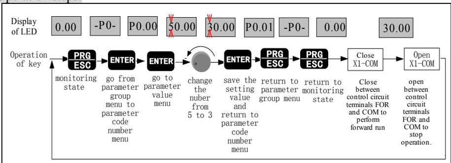
Figure 3-14 Flow chart of running and stop operation by terminal
