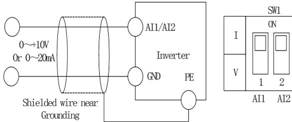
Fig. 2-14 Analogy input terminal wiring diagram
