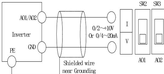
Fig. 2-15 S2R4GB~3004GB/35R5PB Analog output terminal wiring diagram
