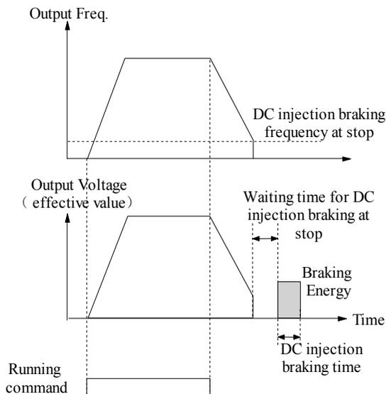
Fig. 5-1-6 DC injection braking
