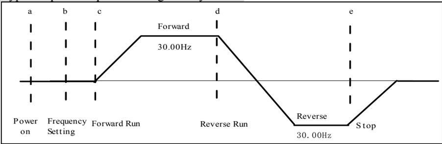
Figure 3-10 Operation sequence by keyboard
