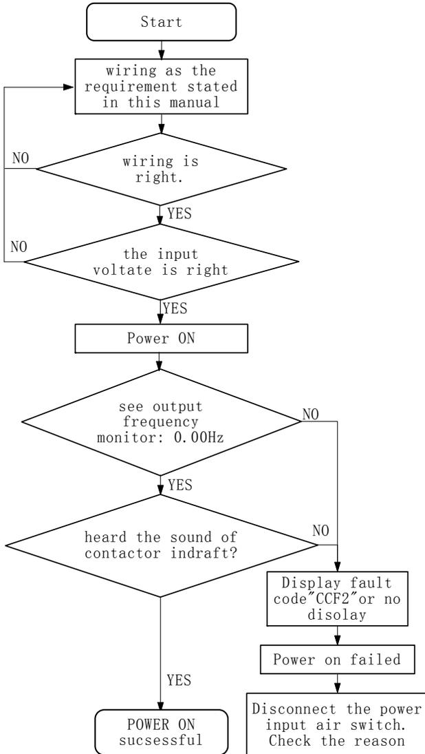
Figure 3-9 Flow chart of the inverter initialization
