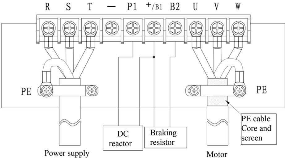
Fig. 2-5 35R5GB/37R5PB~3015GB/3018PB Main Circuit Wiring
