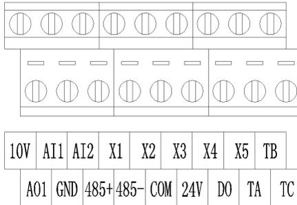
Fig. 2-11 S2R4GB~S2R75GB Arrangement of Control Circuit Terminals
