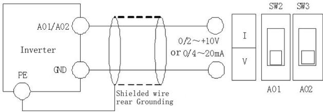
Fig 2-16 35R5GB/37R5PB~3500G Analog output terminal wiring diagram
