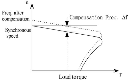
Fig. 5-9-1 Auto slip compensation diagram
