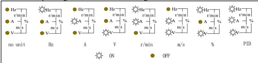
Figure 3-2 Combinations of unit indicator and their means
