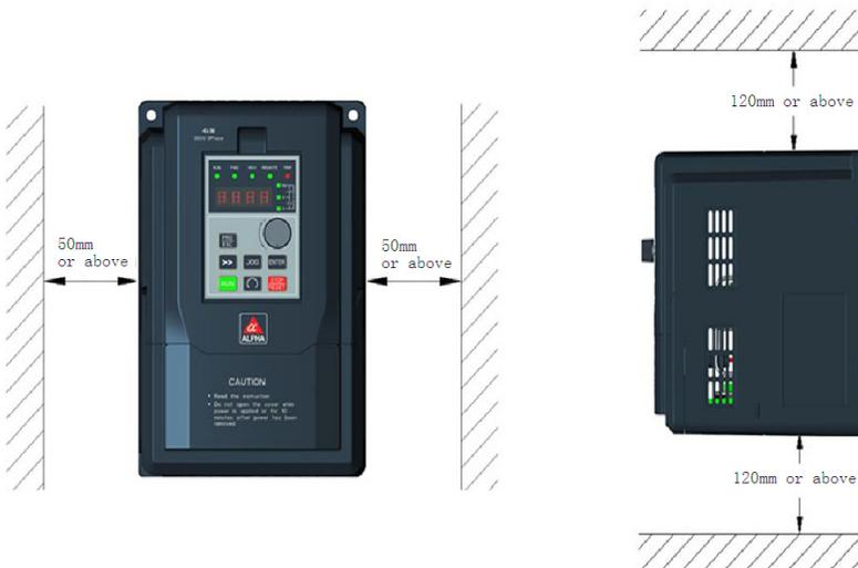
Fig 2-1 Installation Direction and Space
