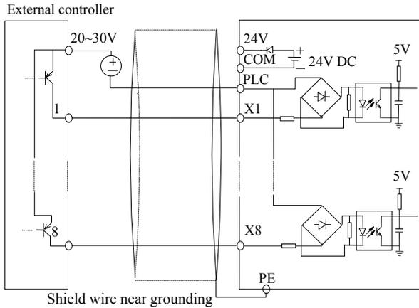
Fig. 2-25 Drain Connection Method(in 3R75GB/31R5PB~3004GB/35R5PB only X1~X5)
