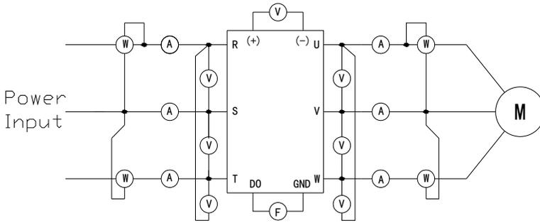
Fig. 8-1 Recommendable Wiring of Main Circuit Electro Measurement
