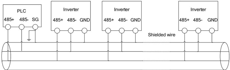
Fig. 2-18 Communication between PLC and the Inverter
