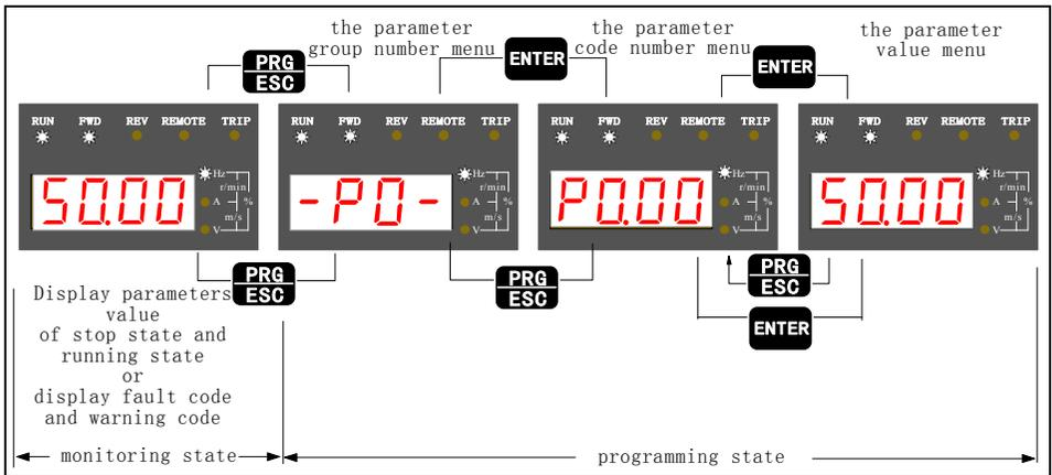
Figure 3-4 Display menus of programming state
