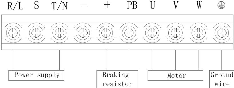
Fig 2-3 S21R5GB~S22R2GB Main Circuit Wiring
