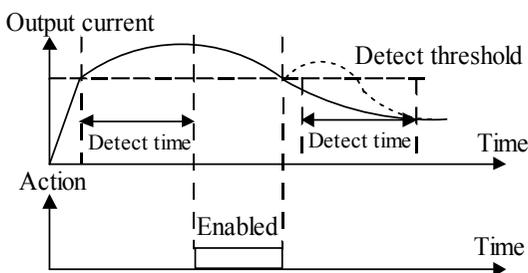
Fig. 5-13-2 Overload pre-alarm function
