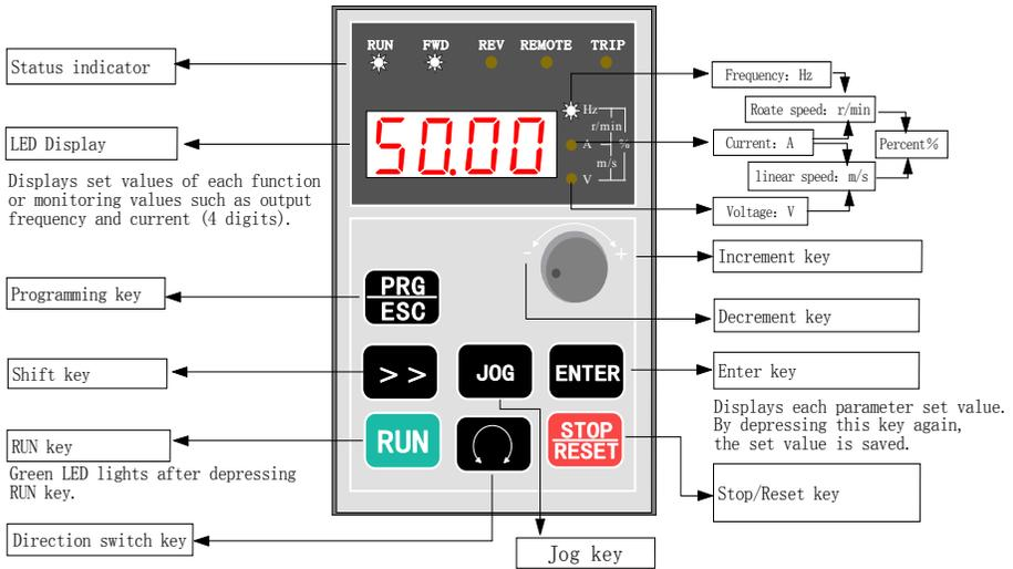
Figure 3-1 Layout and function of Keyboard
