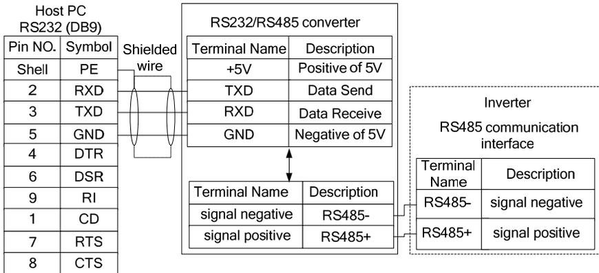
Fig. 2-17 Connection between the inverter and the host PC
