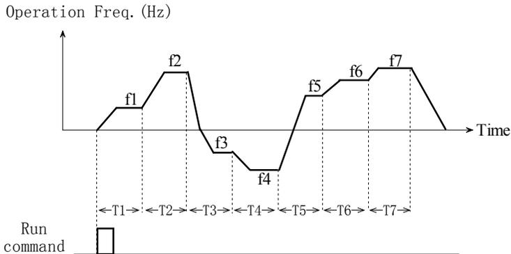
Fig. 5-5-1 Stop mode after single cycle of PLC
