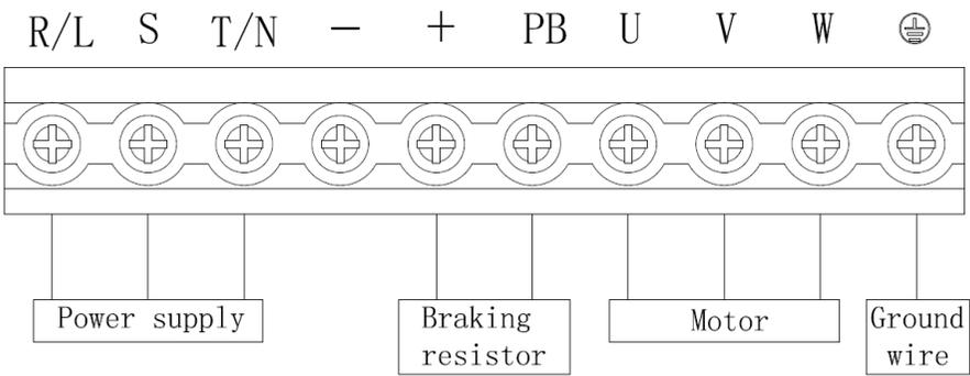
Fig. 2-4 3R75GB/31R5PB~3004GB/35R5PB Main Circuit Wiring
