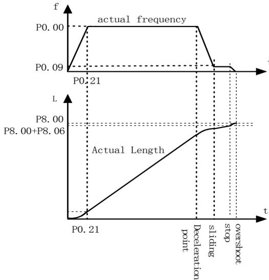
Fig. 5-8-2 Fixed length control diagram 2
