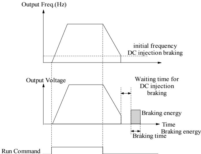
Fig. 5-3-5 DC injection braking
