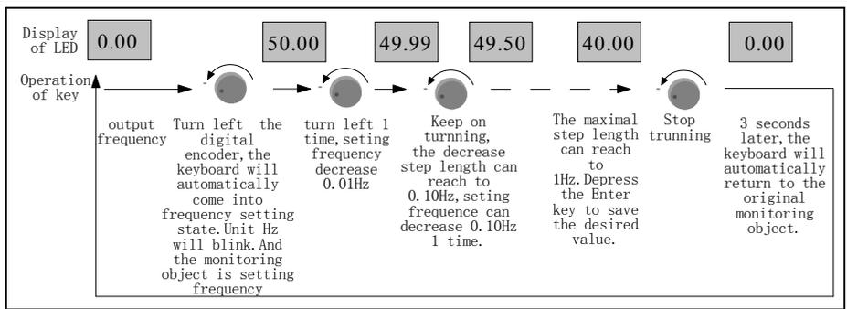
Figure 3-6 Flow chart of frequency setting
