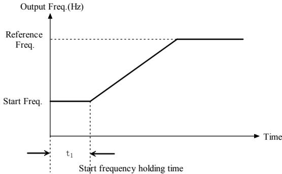
Fig. 5-1-3 Starting frequency and starting time
