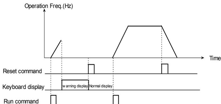
Fig. 5-3-1 Terminal reset
