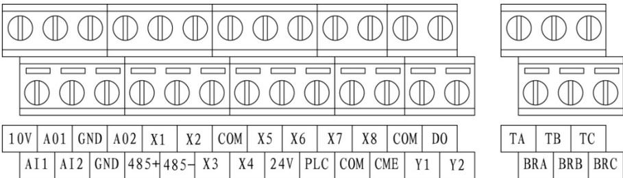
Fig. 2-13 35R5GB/37R5PB~3500GB Arrangement of Control Circuit Terminals
