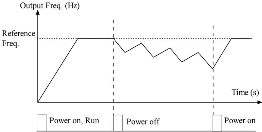
Fig. 5-13-7 Machine does not shut down after power failure
