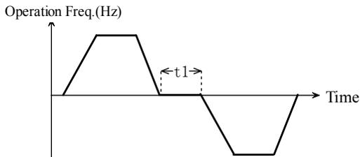
Fig. 5-2-2 FWD/REV switching time diagram
