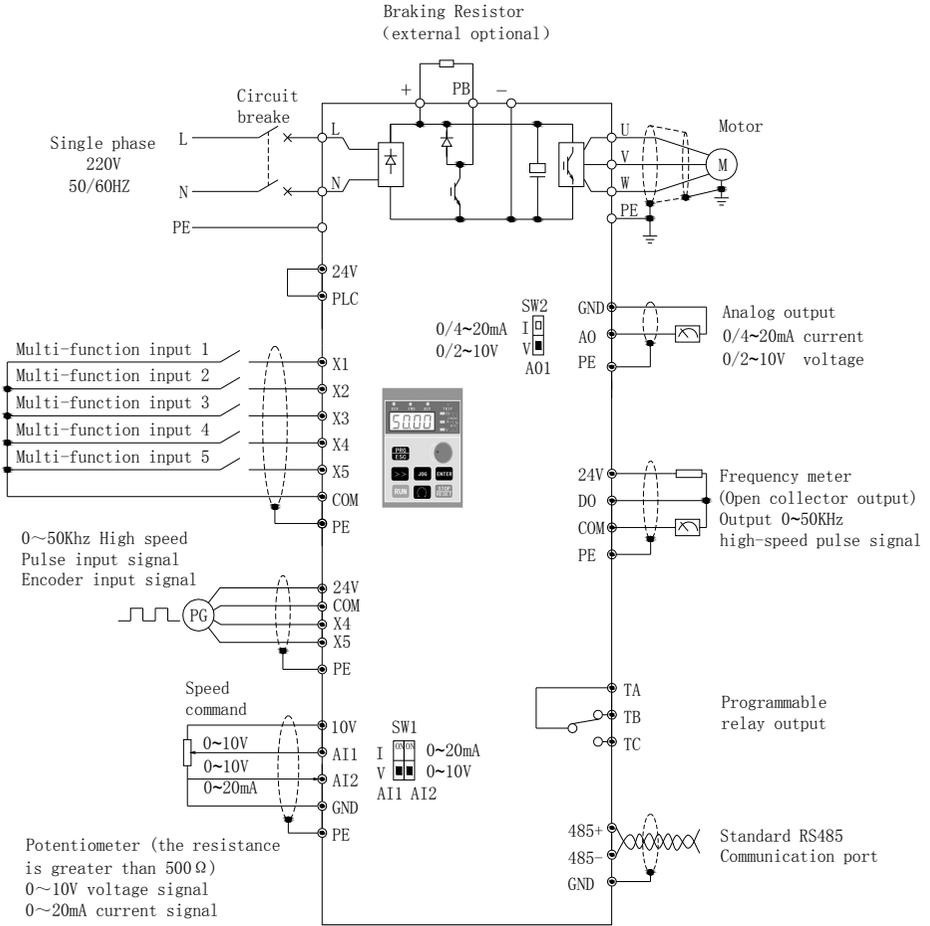
Fig. 2-33 S2R4GB~S22R2GB Wiring diagram (S2R4GB or S2R75GB does not have PLC)
