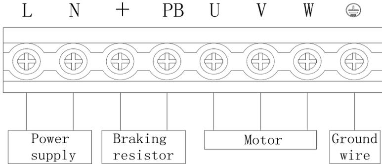
Fig 2-2 S2R4GB~S2R75GB Main Circuit Wiring
