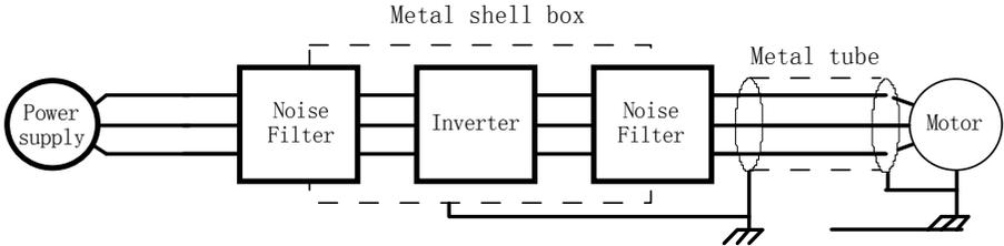
Fig. 2-10 Method to Restrain RFI
