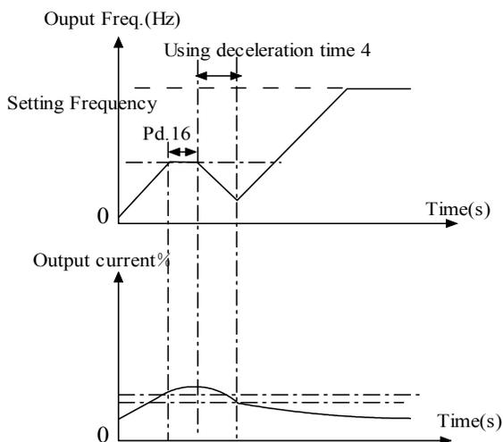
Fig. 5-13-6 Acceleration speed over current
