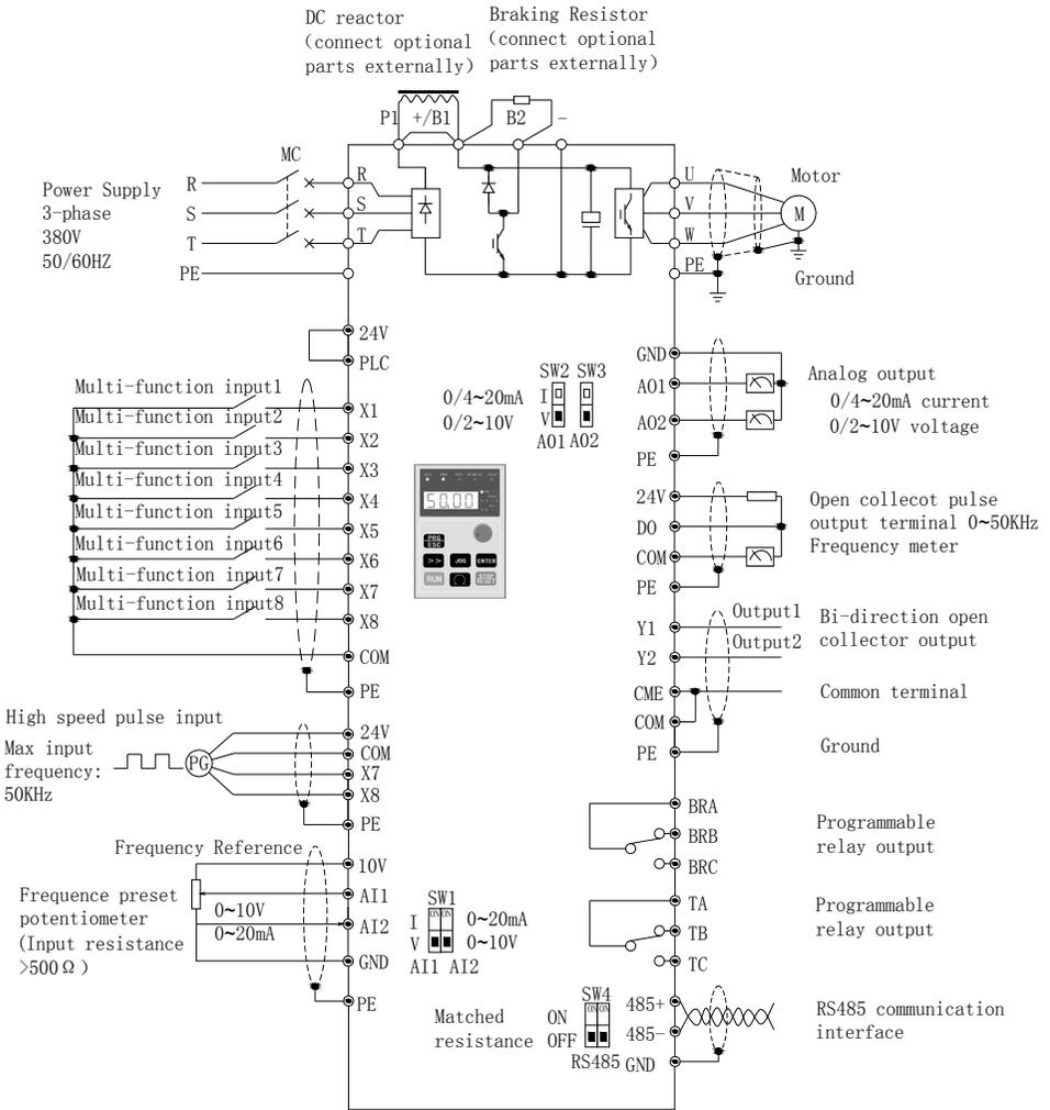
Fig. 2-35 35R5GB/37R5PB~3015GB/3018PB Wiring diagram
