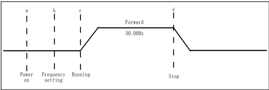
Figure 3-13 Sequence of terminal operation
