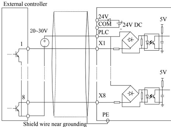
Fig. 2-24 Source connection method by using external power supply (in 3R75GB/31R5PB~3004GB/35R5PB only X1~X5)
