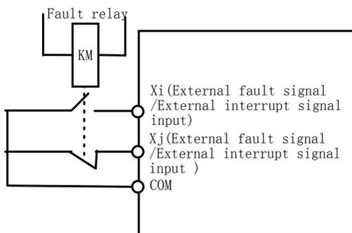
Fig. 5-3-6 Normally open / normally close
