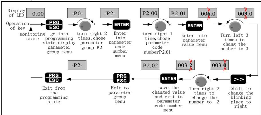
Figure 3-7 Flow chart of parameter setting
