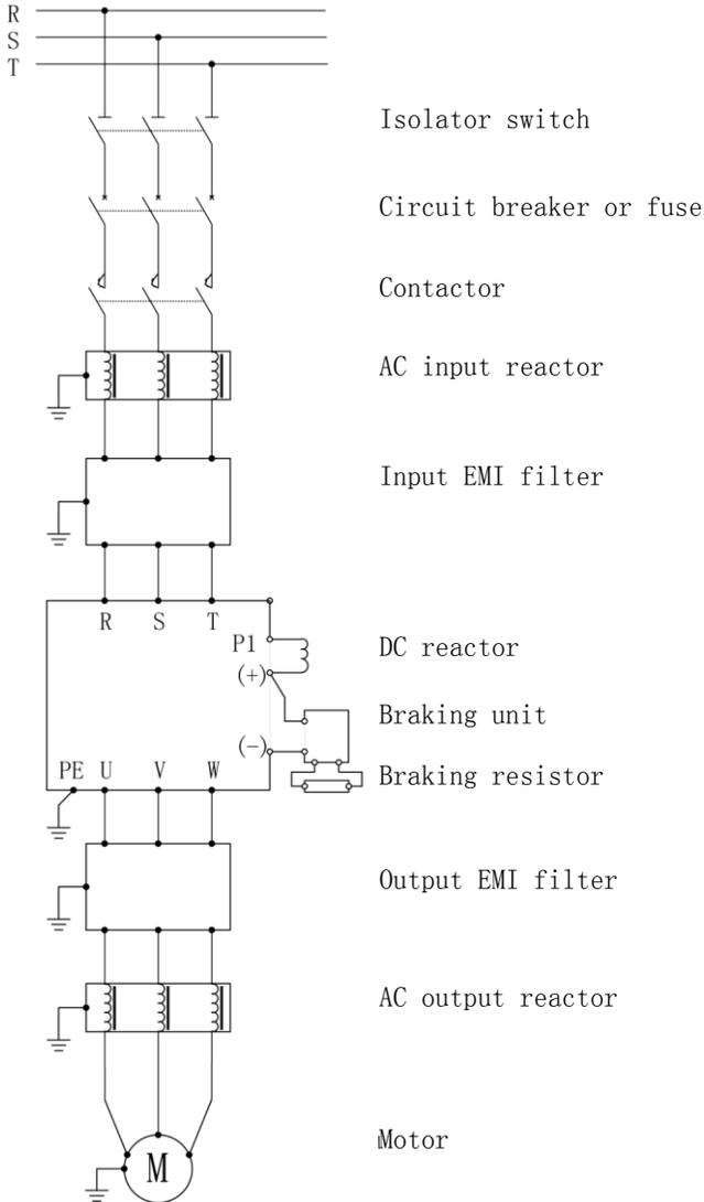
7-1 S2R4GB~3015GB/3018PB Diagrams of Peripheral Equipments
